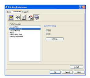
The **Quick Print Setup** feature allows you to quickly choose driver settings. To view settings, simply click your mouse button on the task tray icon. This feature can be set to **On** or **Off** from the Device Options list.
